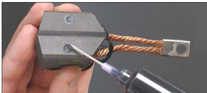
Graphi-Bond™ 551-RN seals sensor in carbon brushes.
