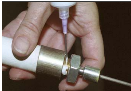
Ceramabond™ 671 used as a high temp threadlocker.
