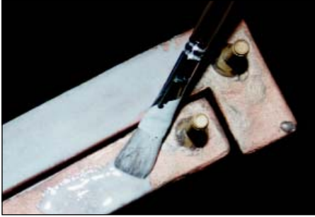
Ceramabond™ 571 coats copper induction heater.
