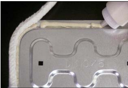
Ceramabond™ 685-N bonds ceramic gasket to metal door.
